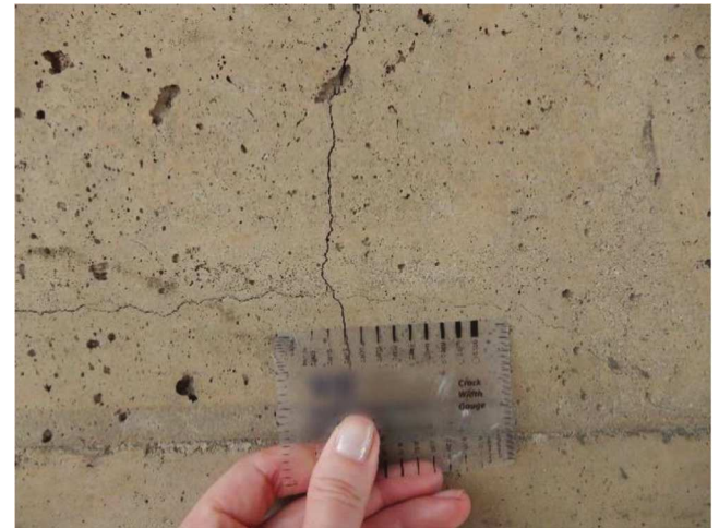
Fig. 4.1.1—Measurement of crack width.
