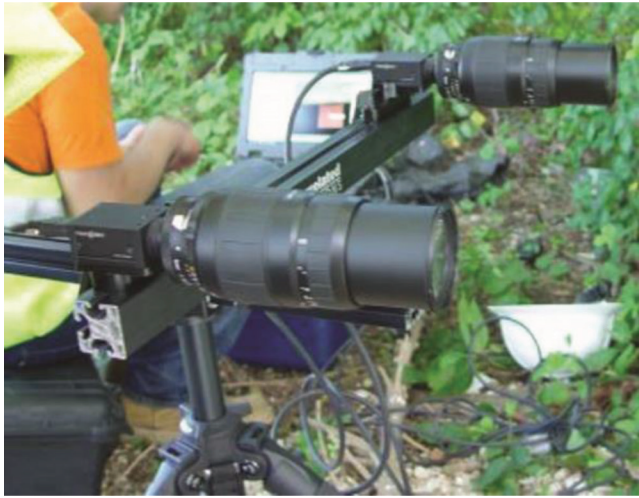
Fig. 4.3.3.1a—Stereo-paired camera setup used during live load testing (Harris 2014).
