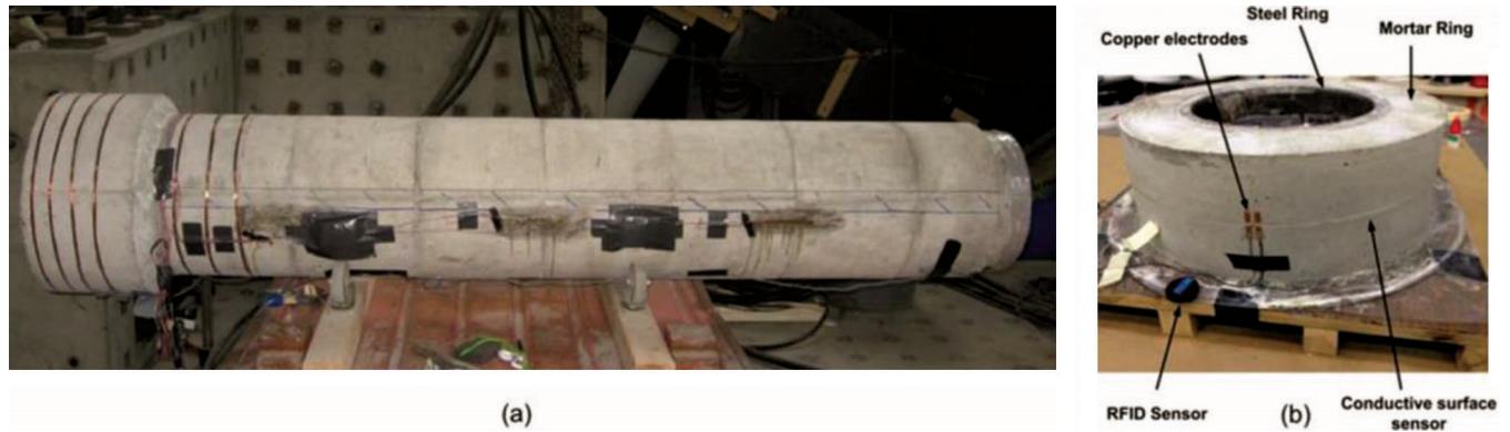
Fig. 4.2.1b—(a) Reinforced concrete pipe segment instrumented with copper metal foil-based one-dimensional CSS (Pour-Ghaz et al. 2011a); (b) restrained ring test instrumented with colloidal silver-based CSS. The response of the CSS is interrogated using radio frequency identification (RFID) technology (Pour-Ghaz et al. 2014).
