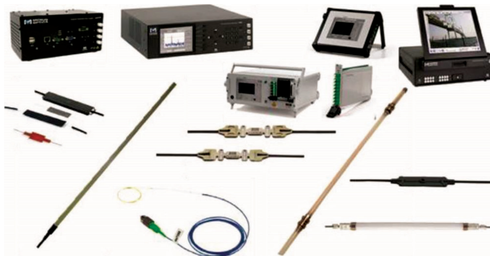
Fig. 4.5.1.4b—Examples of commercially available FBG sensors (both short- and long-gauge) and reading units (courtesy of Roctest/SMARTeC, Micron Optics, and Fiber Sensing) (Glisic 2009).
