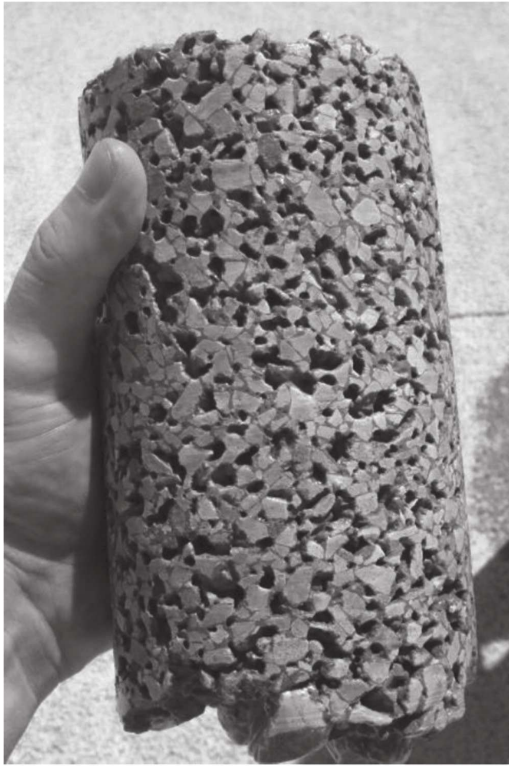
Fig 1.1b—Uniform porosity observed from a core sample (photo courtesy of J. Montgomery).
