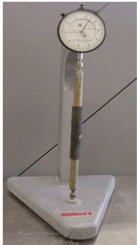
Fig. 4.1.1—Length comparator with standard calibrating rod (ASTM C157/C157M) (Photo courtesy of BASI Construction Chemicals, LLC.)
