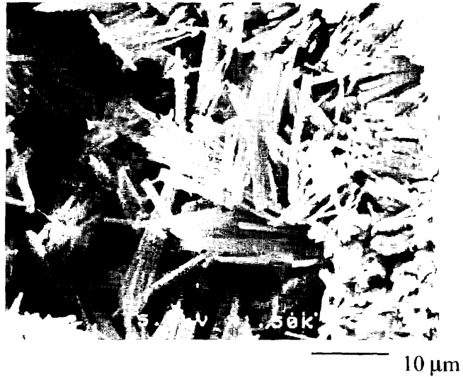
Fig. 14 SEM Micrograph Showing the Deposit at the Joint
