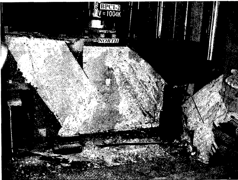
Figure 14: CFRP Fabric Strengthened Inverted Tee Test Specimen Loaded to Failure.
