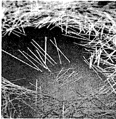
Fig 1A AR Glass Fiber Chopped Strands
