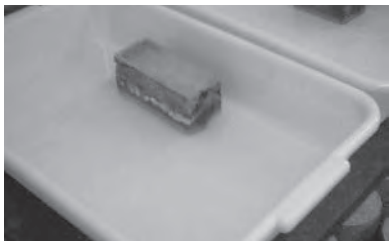
Fig. 3 NaOH crystals in the surface of the realkalised specimens.
