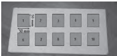
Fig. 4 Coating scheme applied on the premold board.
