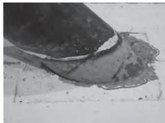
Figure 19 – Failure of connections reinforced with short double-headed studs
