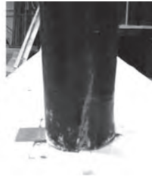
Figure 17 – Failure of verticals in connections reinforced with long double-headed studs
