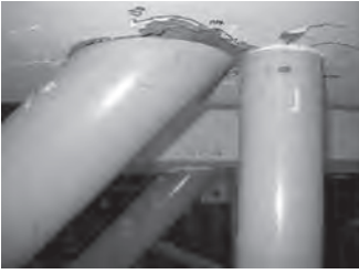
Figure 16 – Failure of diagonals in connections reinforced with long double-headed studs
