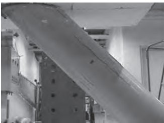
Figure 19 – Failure of connections reinforced with short double-headed studs
