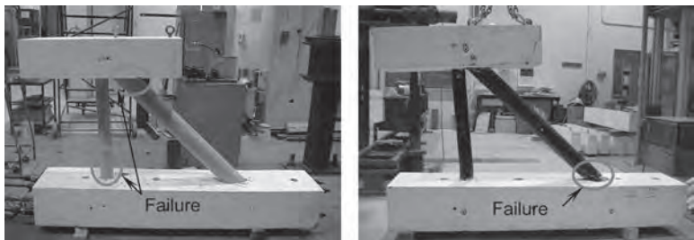
Figure 15 – Failure of connection specimens reinforced with long double-headed studs
