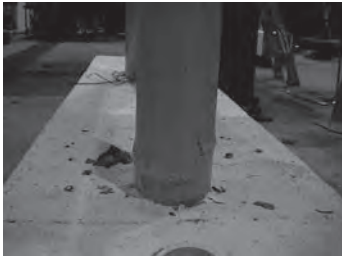
Figure 17 – Failure of verticals in connections reinforced with long double-headed studs
