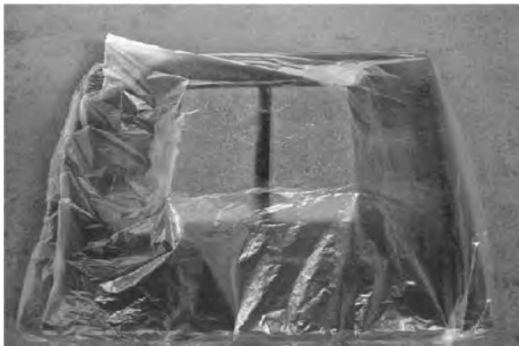
Fig. 2—The situation of packing curing by polyethylene bag after casting.
