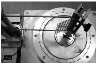
Fig. 8—Bending test with vertical specimen arrangement. [14]
