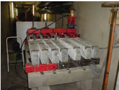
Figure 7—Test set-up for sustained loading (air exposure).
