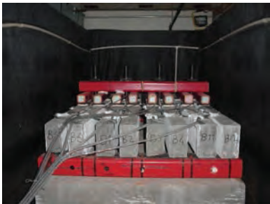
Figure 8—Test set-up for sustained loading (environmental exposure).
