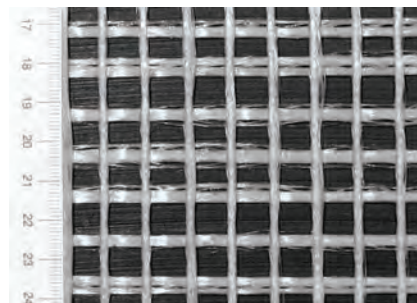
Figure 17: Example of industrial used coated reinforcement textile
