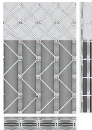
Figure 10: CAD model of a warp knitted textile structure
