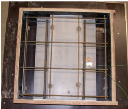
Figure 17 — Test sample for the fire resistance test
