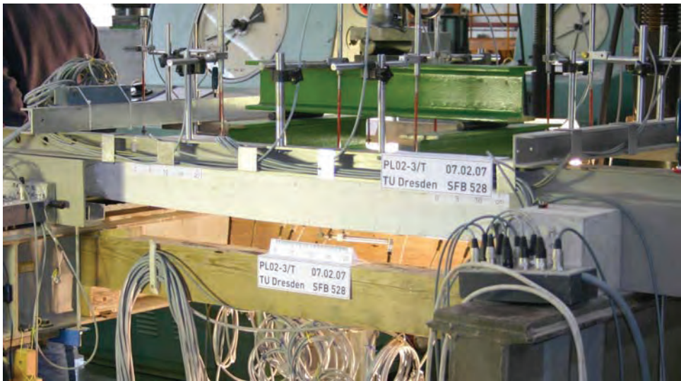
Figure 1 — Test set-up of TRC-strengthened RC-slabs
