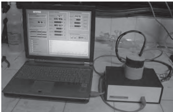
Fig. 4–Sensor (embbeded in mortar) and adquisiton data system for measurements on concrete structures.
