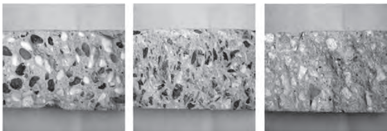
Fig. 3 – Fracture surfaces (splitting tests).
