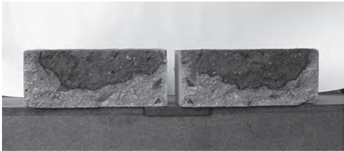
Fig. 4 – Water penetration profile on both halves of one of the assessed specimens.
