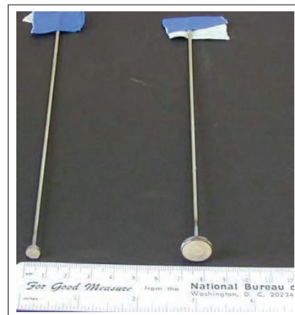
Fig. 2(b) - Pore pressure gages
