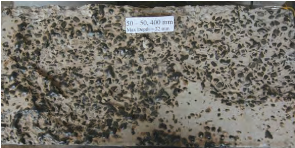
Fig. 10 – Underside of 50/50, 400 mm specimen.
