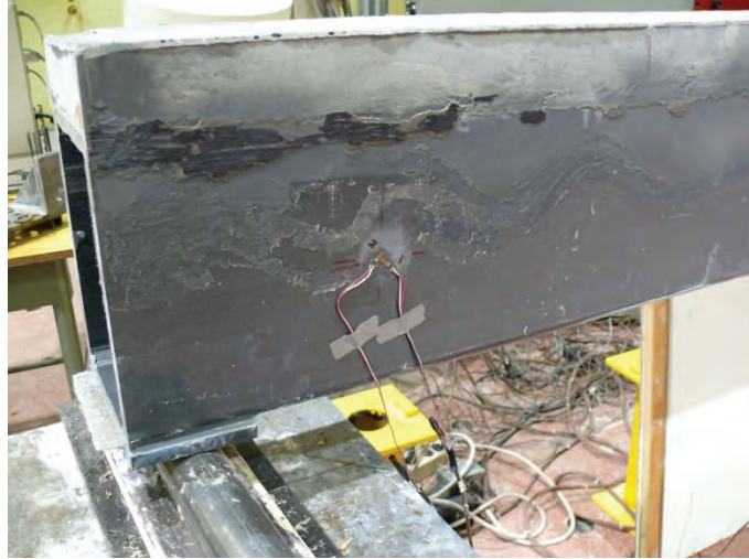
Figure 10 — Bearing plate support of Beam 1
