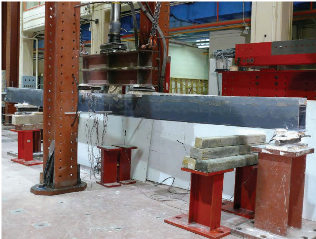
Figure 8 — Test arrangement for Beam 1
