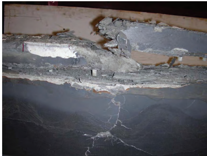
Figure 15 — Failure of Beam 3
