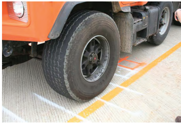
(b) Truck Wheel Positioned Over Deck Target (Strain Gauge in this Case)
