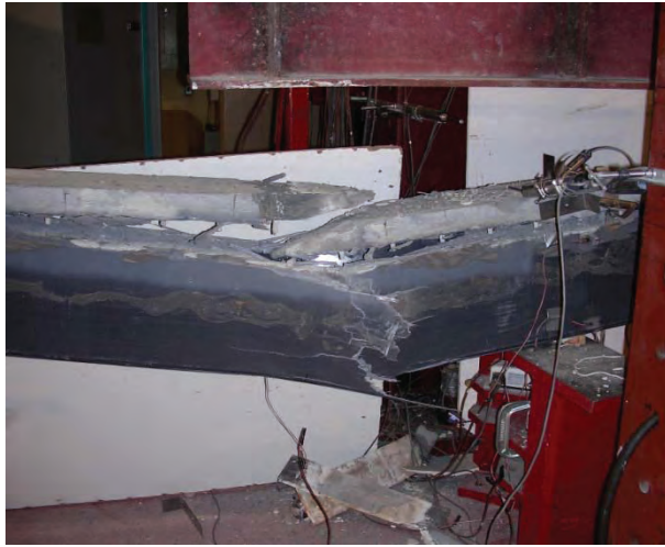
Figure 13 — Failure of Beam 2
