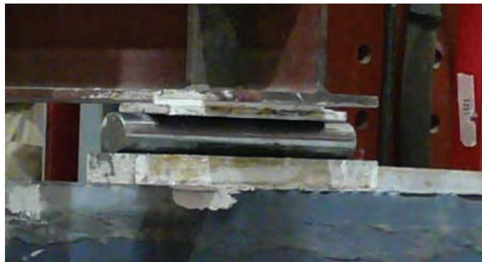
Figure 14 — Loading plate for Beam 3
