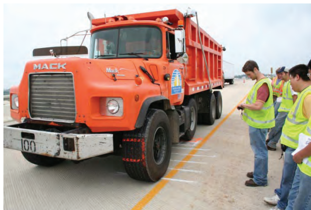
(c) Truck Positioned at Last Deck Target in Loading Protocol with Pause
