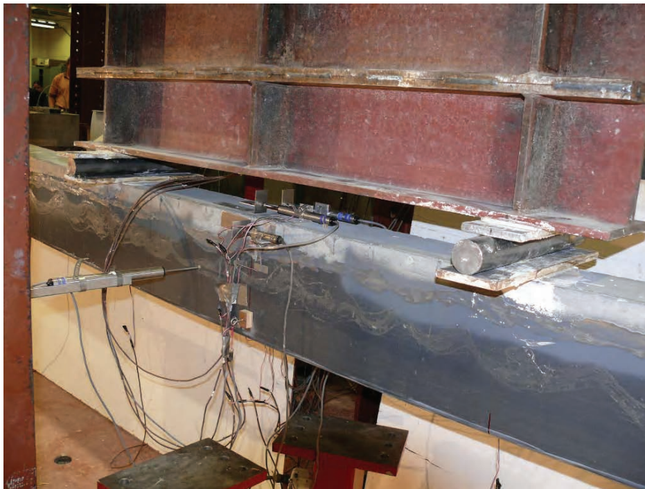
Figure 7 — Instrumentation of the beams at the mid-section
