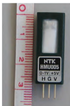
Photo 3 –Ceramic RH sensor (with temperature-correction circuit)
