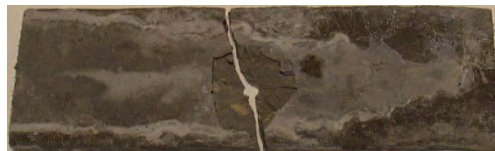
Figure 2-- Failure modes of extruded composites (nail exit face).
