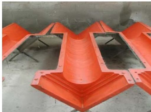
Fig. 26—Molds for GFRC permanent column forms.
