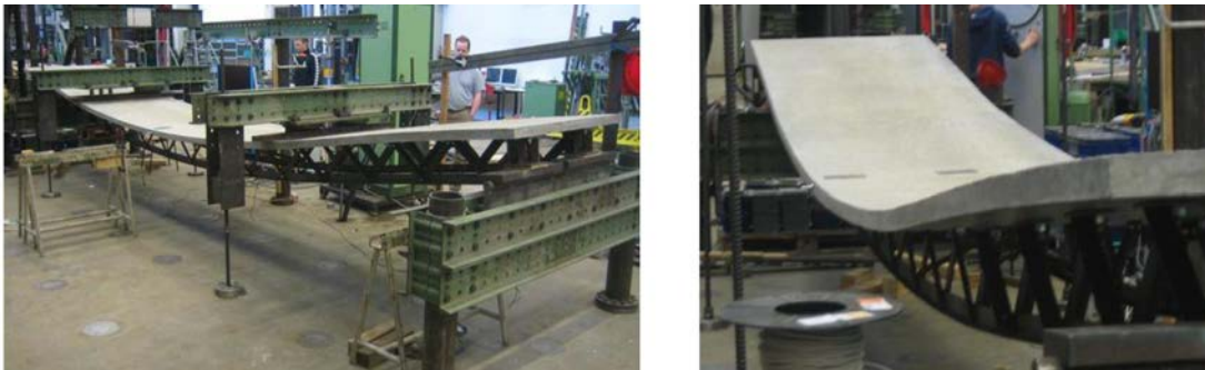
Fig. 11—Deformed shape of Specimen S2 during (left) and after (right) ULS loading.
