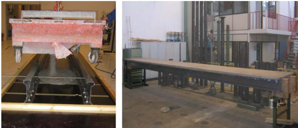
Fig. 4—Integrally cast floor panel during fabrication and prior to testing.
