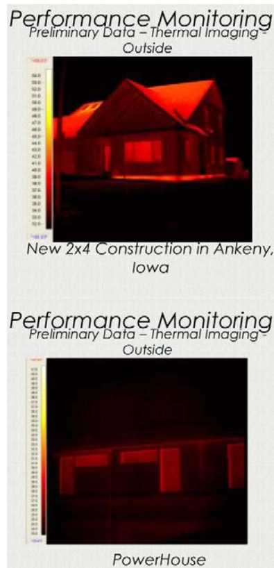
Fig. 17—Thermal imaging comparison of conventional house and GFRC house.
