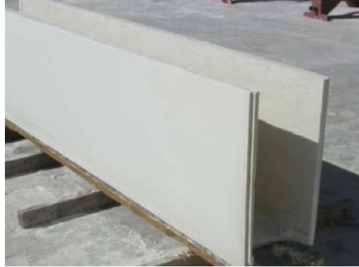
Fig. 25—Finished GFRC beam form.
