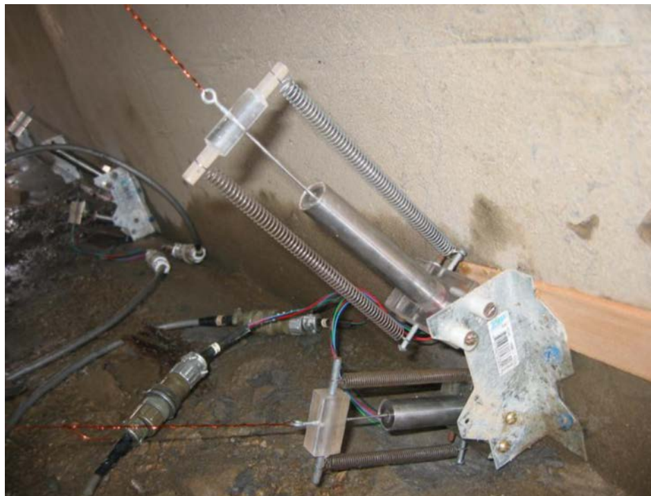
Fig. 10—Example of DCDT mounted to base of arch unit leg to measure vertical and horizontal displacements.
