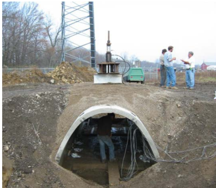
Fig. 8—End elevation of full-scale load test setup.
