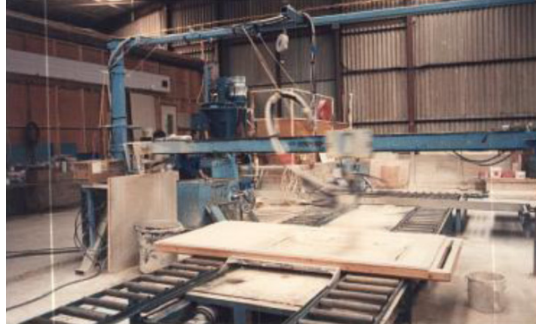
Fig. 19—Semi-automatic reciprocating spray machine.
