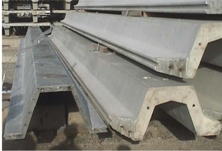
Figure 11—Prestressed sheet piles cast with SCFRC (left: C90/105) and conventional concrete (right: B55/67 concrete with additional bar reinforcement)
