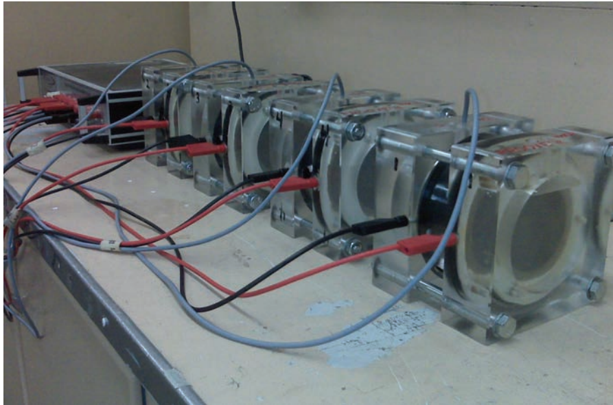
Figure 1—The rapid chloride permeability test setup.
