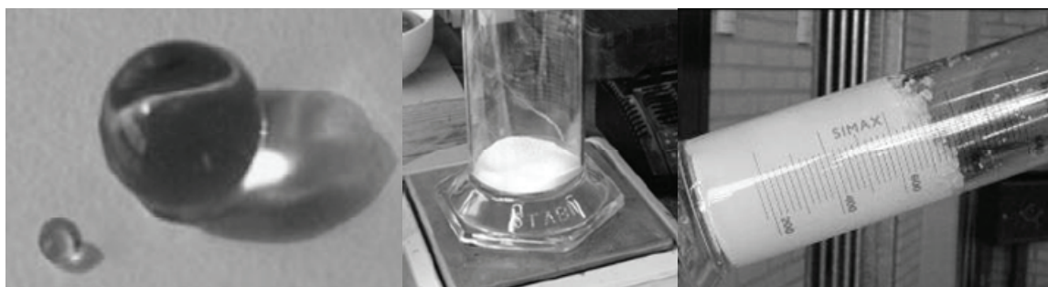
Figure 1—From left to right two Super Absorbent Polymers, one unsaturated and one saturated (Jensen and Hansen 2001), 25 grams of unsaturated polymers and 630grams of water absorbed by 25 gram polymers.
