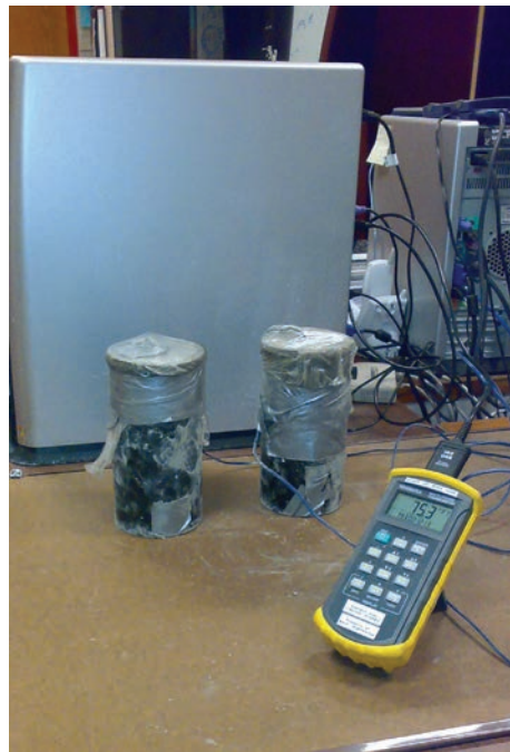
Figure 1—The rapid chloride permeability test setup.
