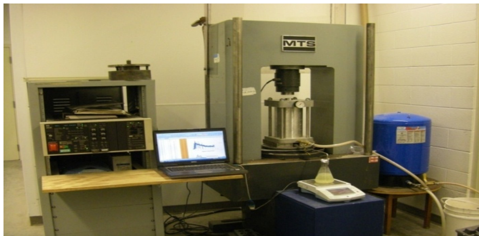
Figure 4. Measuring the Water Permeability under Stress
