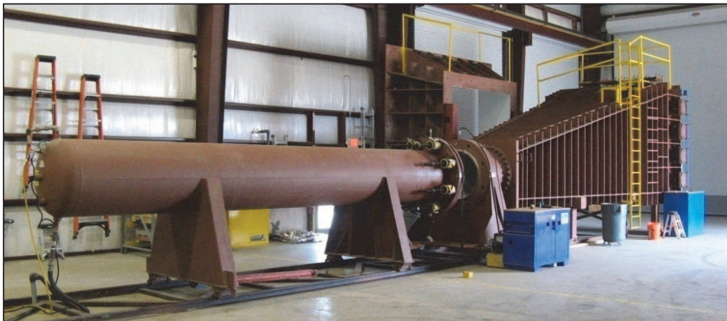
Figure 2 — BakerRisk Large Shock Tube
