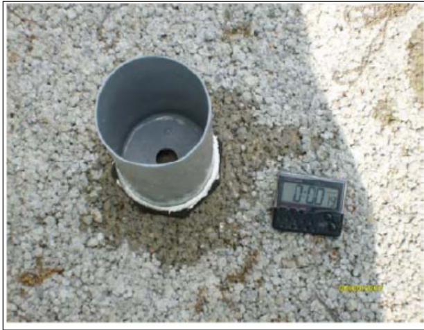
Figure 2 – surface hydraulic conductivity/infiltration apparatus
