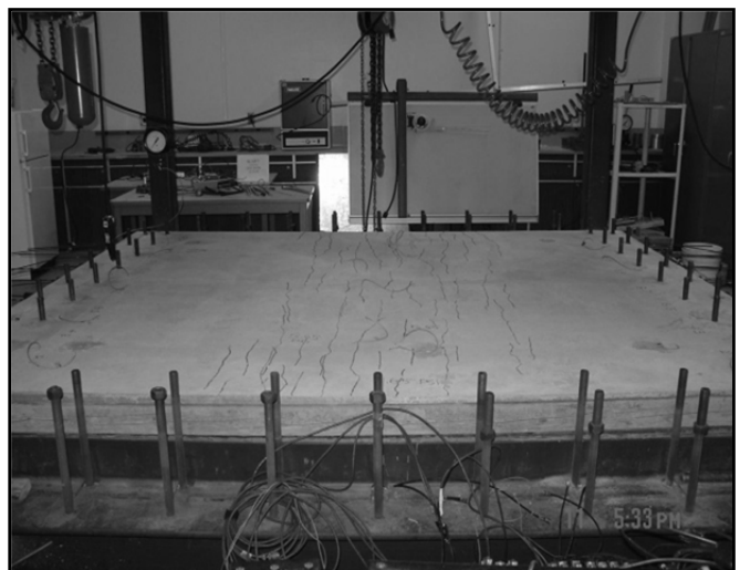
Photo 8- PTS-1(PTS-2&6 similar) Cracking-Ult-Load (at CSUF)
