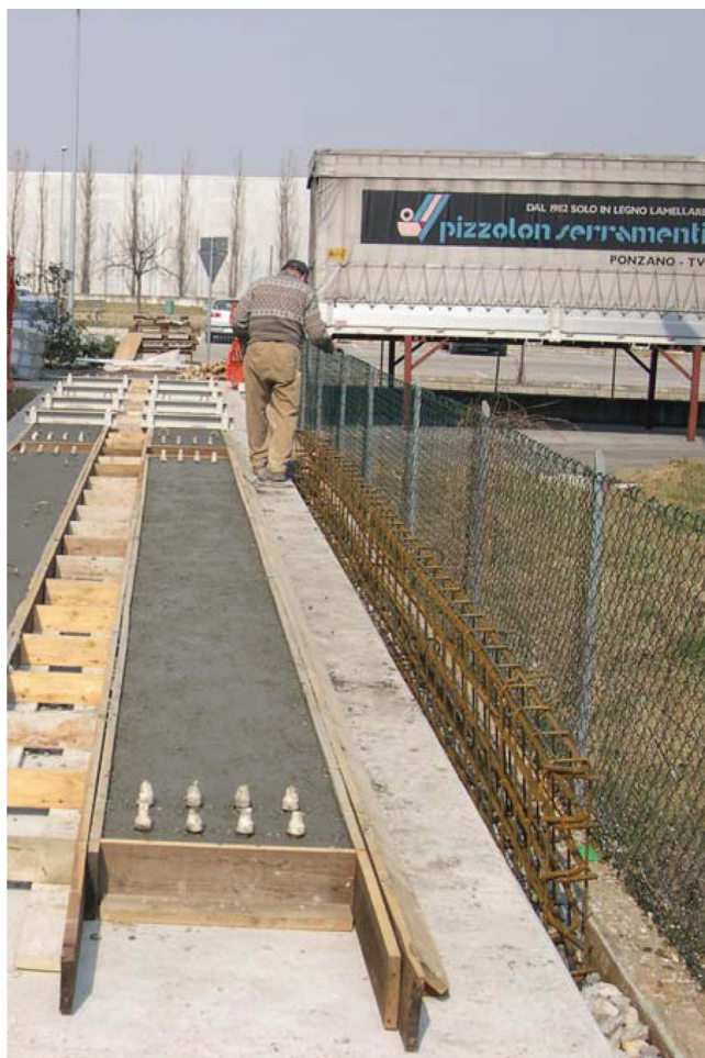
Fig.1 – Field tests on restrained drying shrinkage of concrete slabs 8 m long, 400 mm wide and 60 mm thick (8.75-yd long, 16-in wide and 2.3-in thick).
