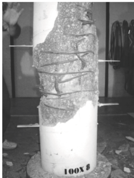
Fig. 4—Typical Specimen at Failure
