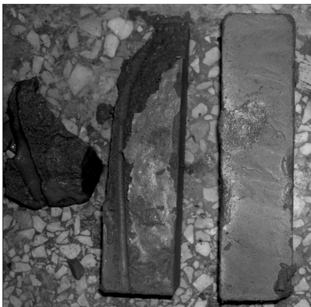
Fig.5 Reference sample's shape change after bring back from negative to positive temperature
