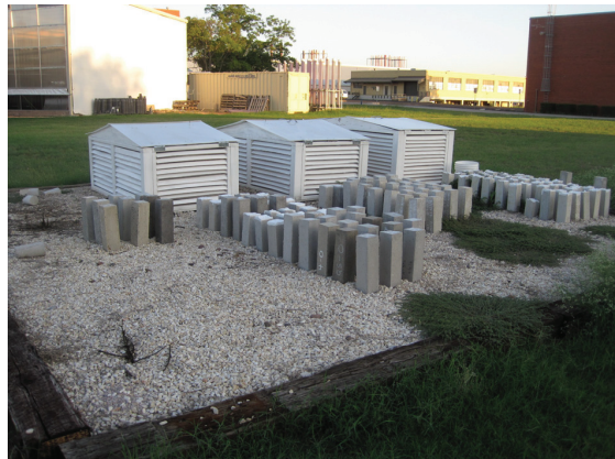
Figure 1—Outdoor natural carbonation exposure site located in Austin, TX.
