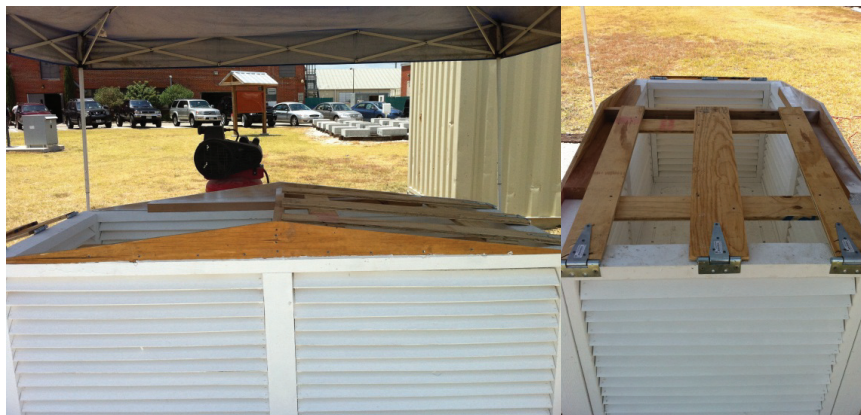
Figure 2—a) Wooden slat strips used in the long span of the Stevenson screen. Each slat was cut to fit inside each wall panel, b) long span wooden frame illustrating the isosceles triangles at the ends, c) final design of Stevenson Screen frame
