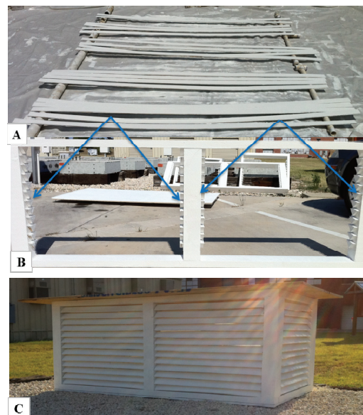
Figure 2—a) Wooden slat strips used in the long span of the Stevenson screen. Each slat was cut to fit inside each wall panel, b) long span wooden frame illustrating the isosceles triangles at the ends, c) final design of Stevenson Screen frame
