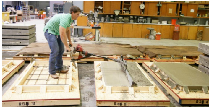
Figure 4- Preparation of the slabs. The tolerance of the reinforcement vertical location seems to be the wider among other dimensional tolerances
