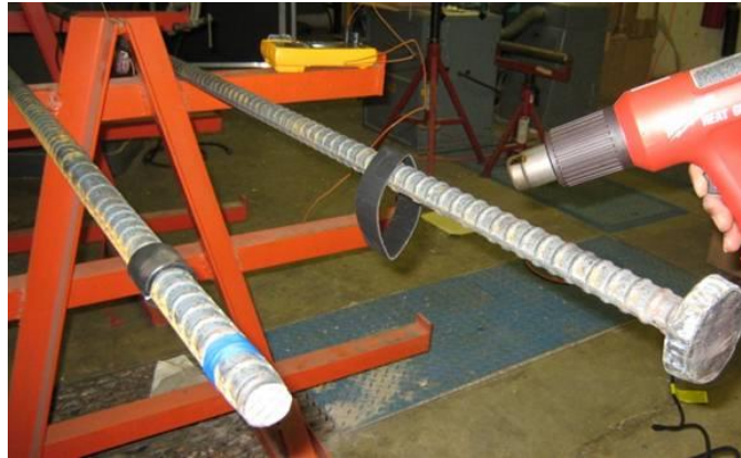
Fig. 5–Polyolefin shrink tube before (right) and after (left) heat treatment.
