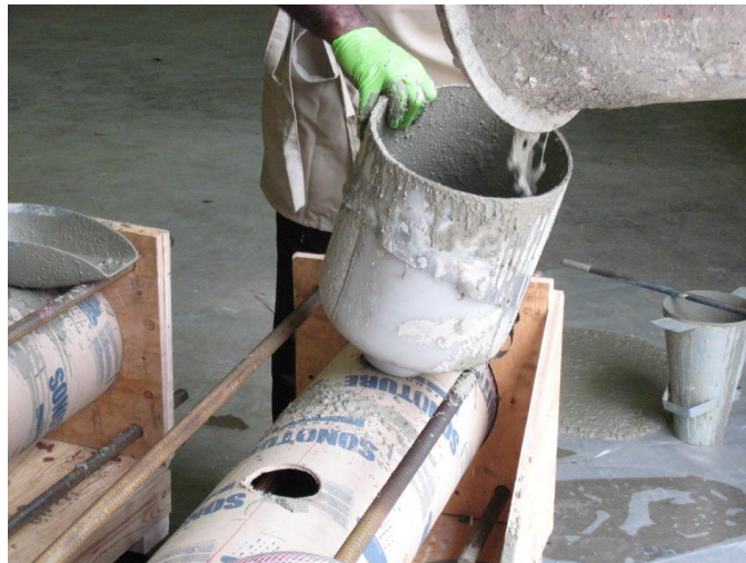
Fig. 6–Concrete placement in cylindrical forms.
