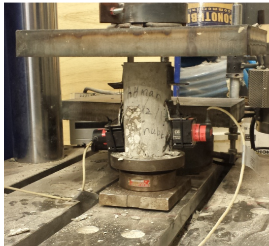
Figure 2 -- Compression test setup
