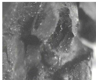
Figure 3: Typical tire rubber particle at 20X magnification (Reda Taha et al., 2008).
