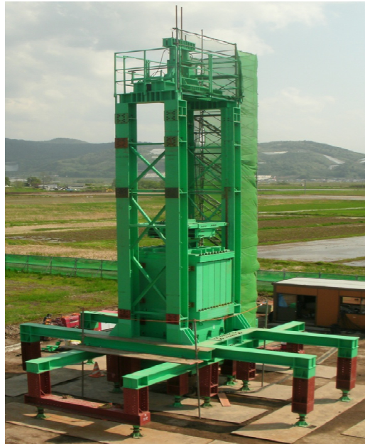
Figure 17 —Rapid pile load test (photograph courtesy: Jibanshikenjo Co. Ltd.)
