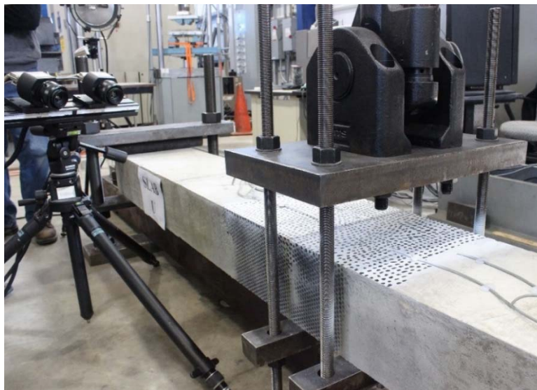
Figure 9 – Test setup for flexural crack width slab specimen
