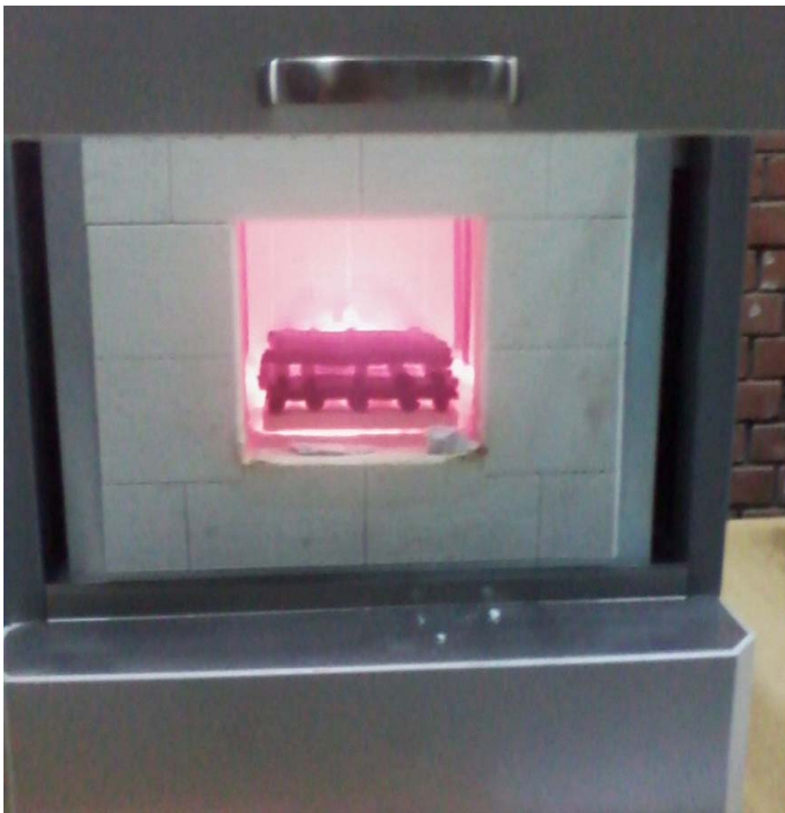
Fig. 1 - Rod-shaped raw meal in production furnace.
