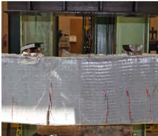
The GFRP wrapped beam after failure
