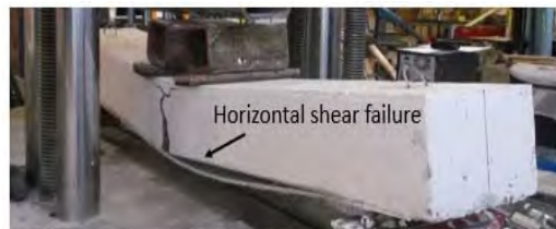
(c) Horizontal shear failure of GFRP ribs from base in S4 and S8
