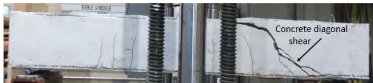
(d) Concrete shear failure (diagonal) in S5 and S9
