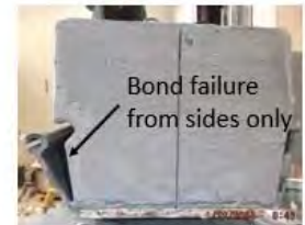
(b) Concrete shear failure (diagonal) with bond failure in S2 and S3
