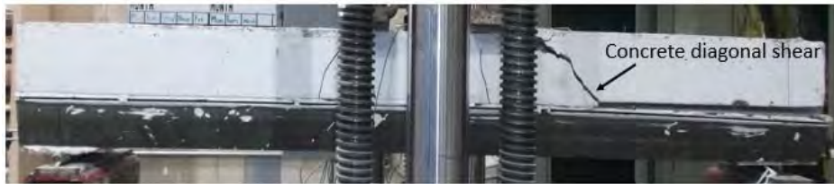
(b) Concrete shear failure (diagonal) with bond failure in S2 and S3
