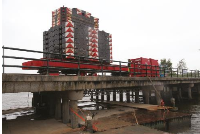
Figure 10 — Use of steel spreader beam, hydraulic jacks, and counterweights in the test on the second span for the Ruytenschildt Bridge.
