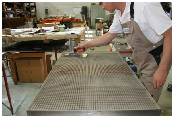
Figure 3 — Manufacturing of specimen, here: application of the first layer of reinforcement (photo: Karoline Holz)
