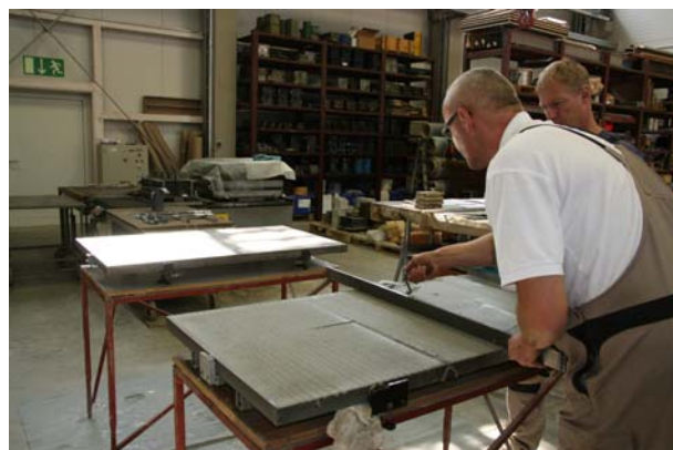
Figure 2 — Manufacturing of specimen, here: application of the first concrete layer into the formwork (photo: Karoline Holz)
