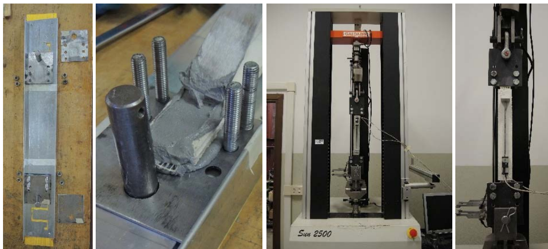
Figure 5 — Detail of the assembly template for tensile tests (left), detail of the bonding with quick-setting resin (centre-left) and mounted test set-up (centre-right and right)
