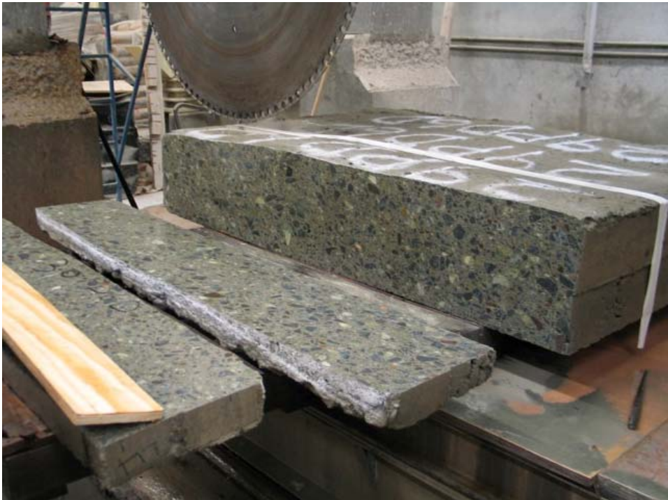
Figure 6 – Sawcutting test panel into test blocks and elements for core drilling
