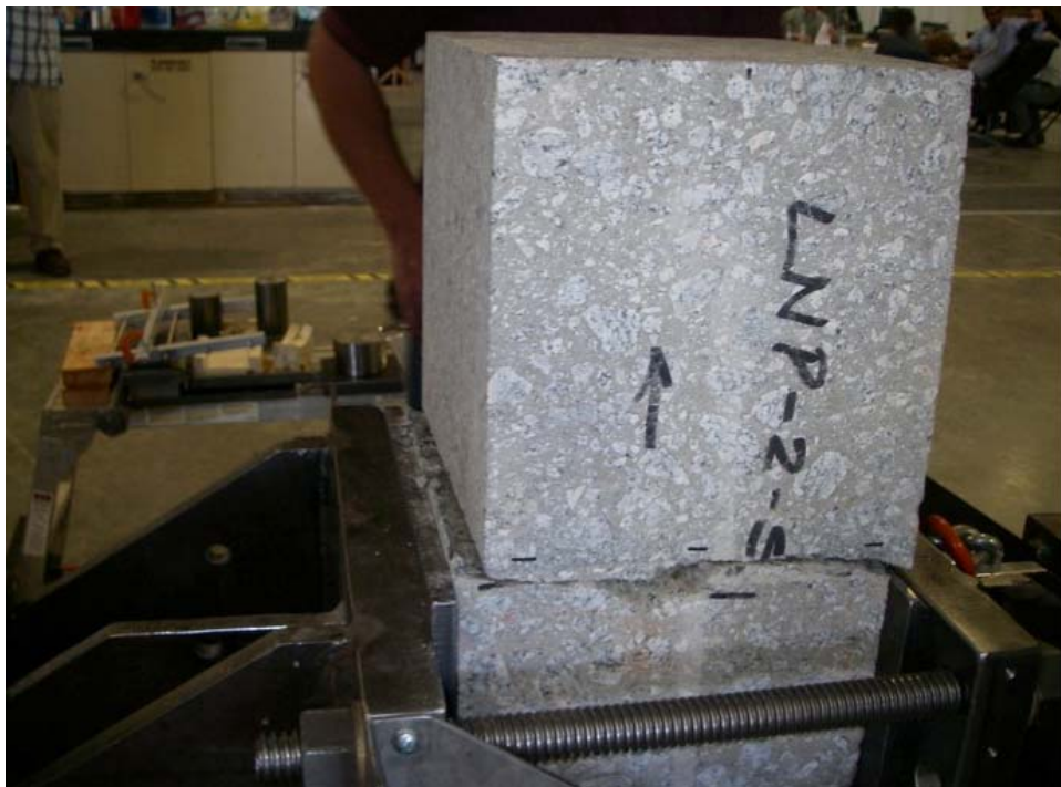
Figure 10 – RCC block after completion of shear test at a lateral displacement of 0.5 inches (12mm)
