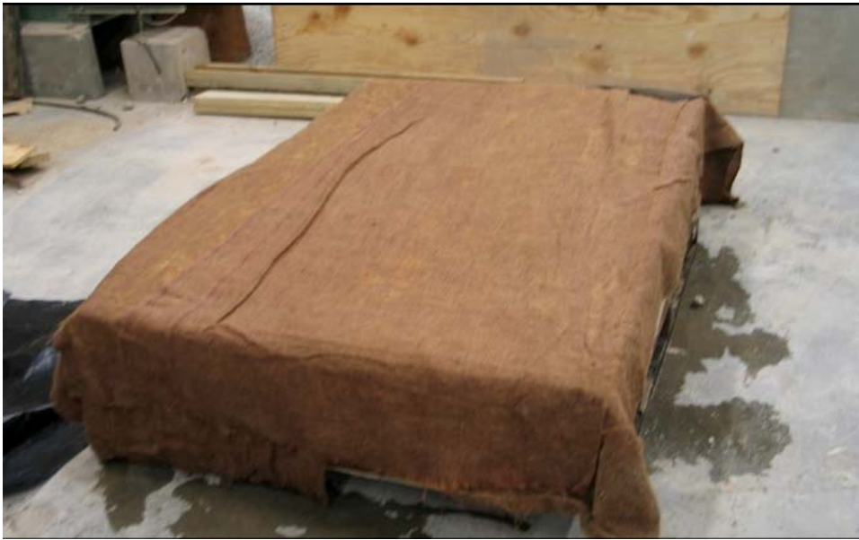
Figure 5 – Continuous wet curing of complete test panel
