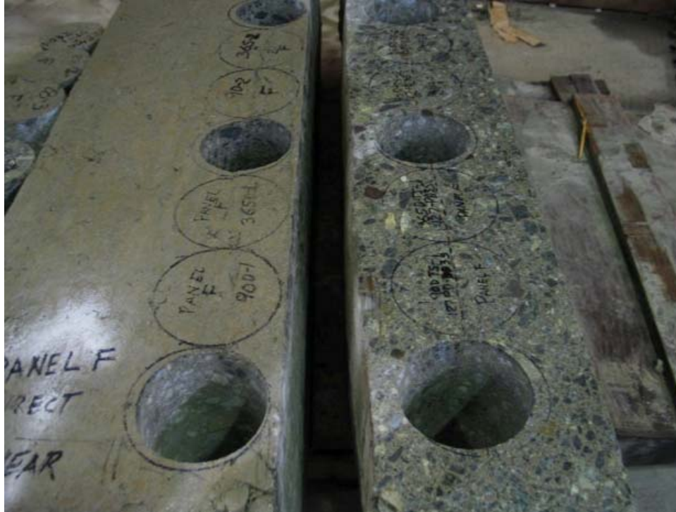
Figure 7 – Core locations for tensile testing specimens
