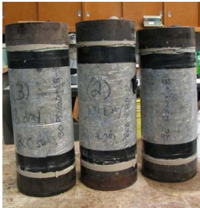
Figure 8 – Prepared specimens for direct tensile testing
