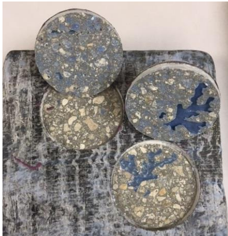
(b) Water resistance samples' failure mode
