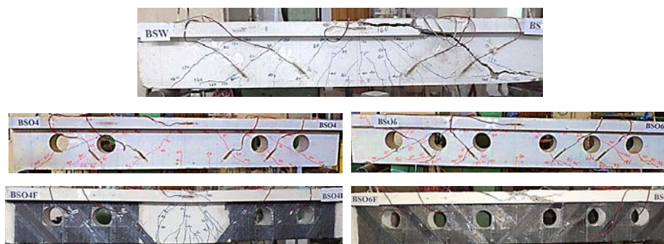
Fig. 6—Crack patterns for static tested beams
