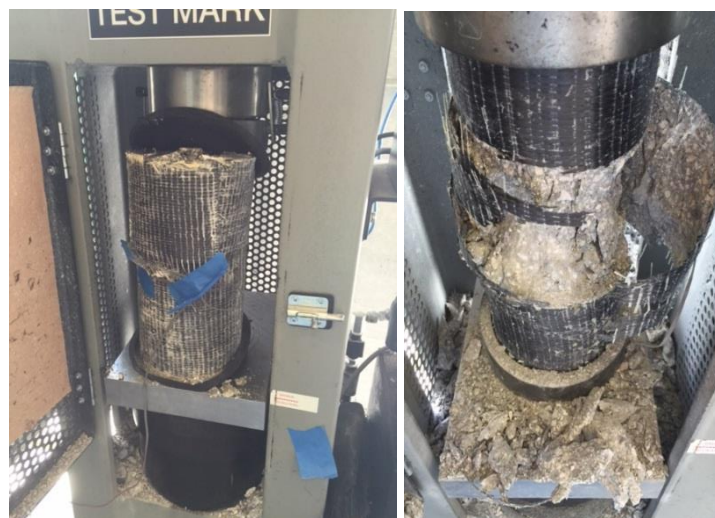
Figure 4 – Typical failure modes during compression testing
