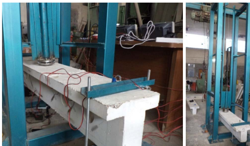
Fig. 5—Experimental set-up for the dropping mass impact test
