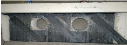
Fig. 2—Alignment of CFRP fabric
