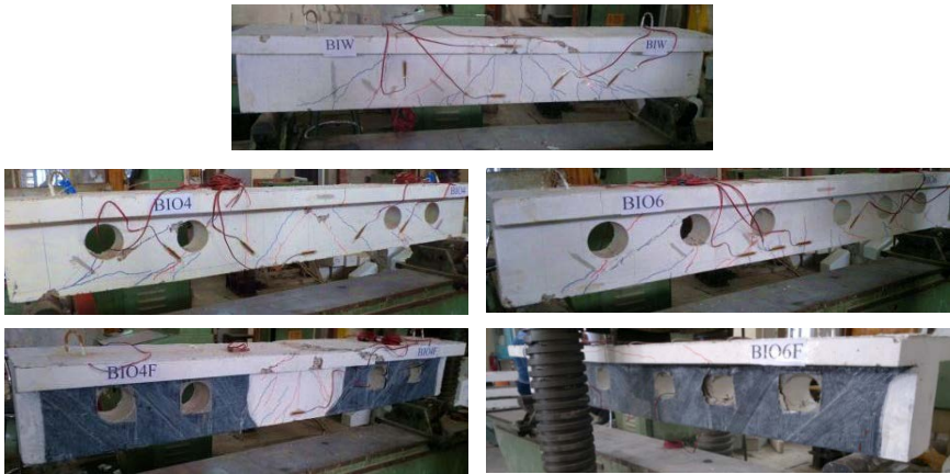
Fig. 15—Crack patterns for impact tested beams after static tests
