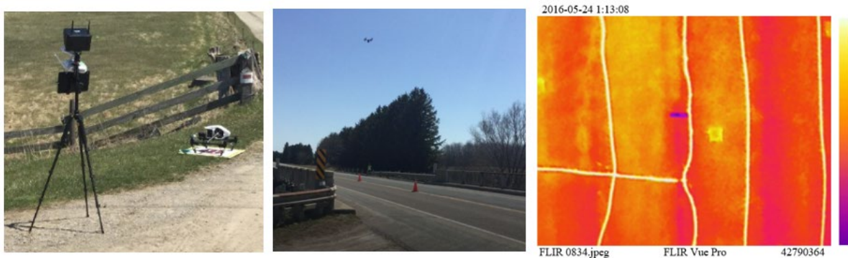
Figure 3 -Setup of UAV-borne thermal system and a snapshot during flight over bridge (2).
