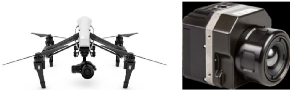
Figure 2 -Aircraft (Inspire 1 Pro) and thermal camera (FLIR Vue Pro) utilized in this study.
