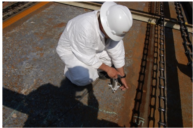
Figure 7 – Impact-Echo testing: Identify internal defects
