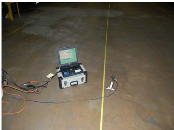
Figure 7 – Impact-Echo testing: Identify internal defects
