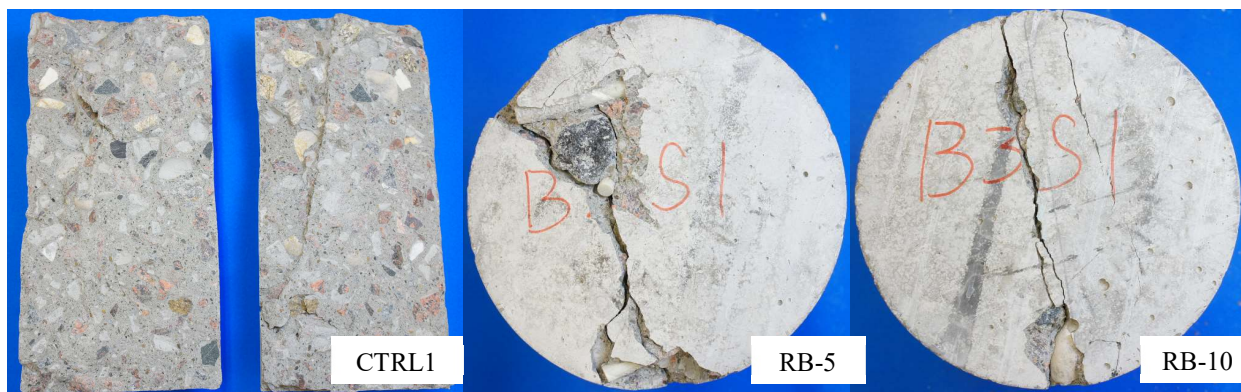
Figure 2- Representative Concrete specimens after splitting tensile strength tests in the first phase of the experiments, investigating rebar needles.
