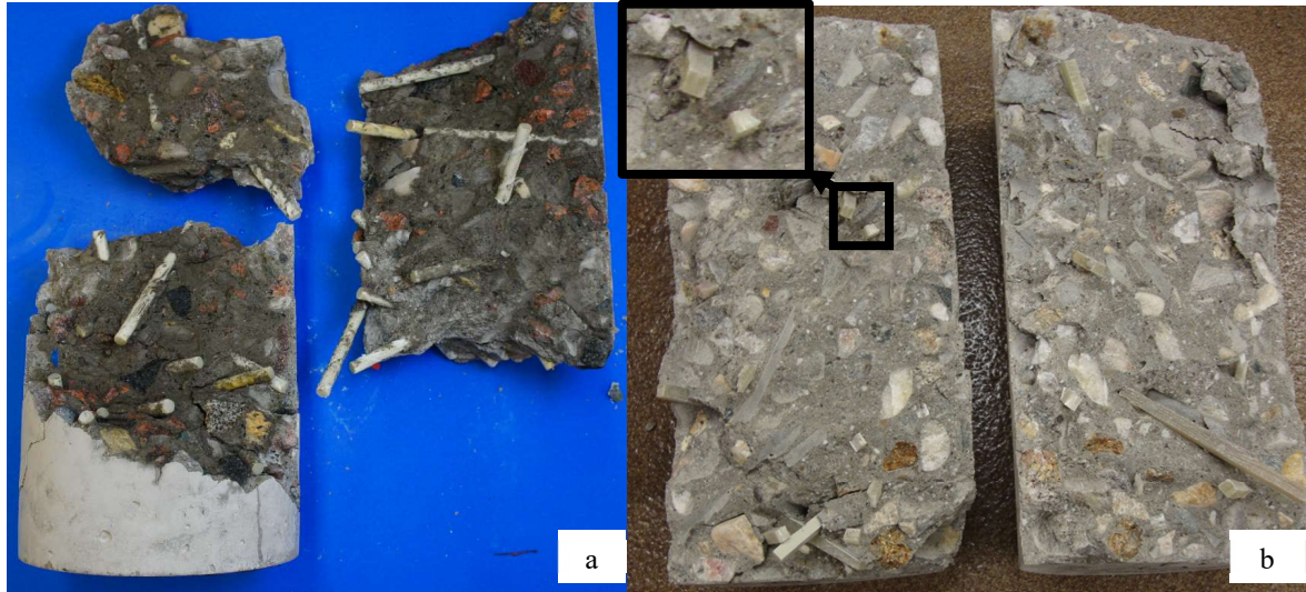
Figure 5— (a) GFRP rebar needles and (b) wind blade needles in representative specimens tested for measuring splitting tensile strength. The specimens were opened manually after the tests were completed. In both specimens, 10% of coarse aggregate is replaced by needles.
