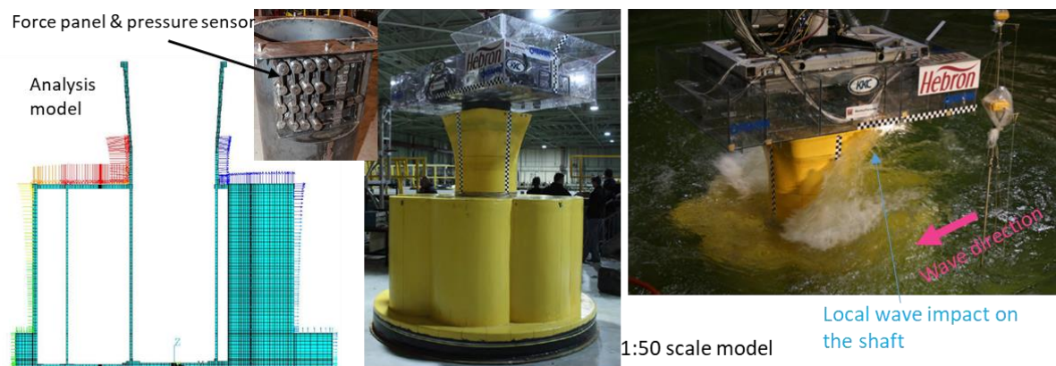
Fig. 2 – Determination of wave-structure interaction on a GBS
