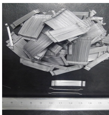
(a) 35mm hooked end steel fibre
