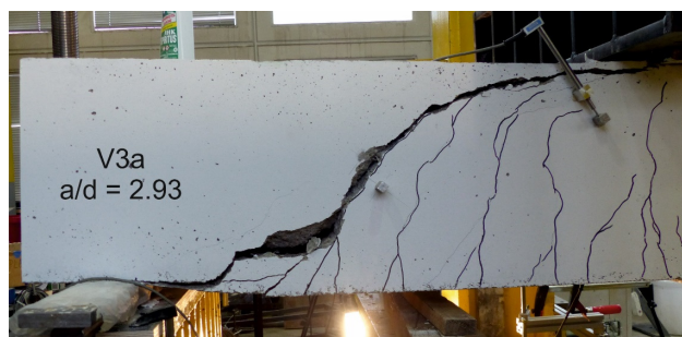
Figure 15 –Shear-compression failure of specimen V3a [60]
