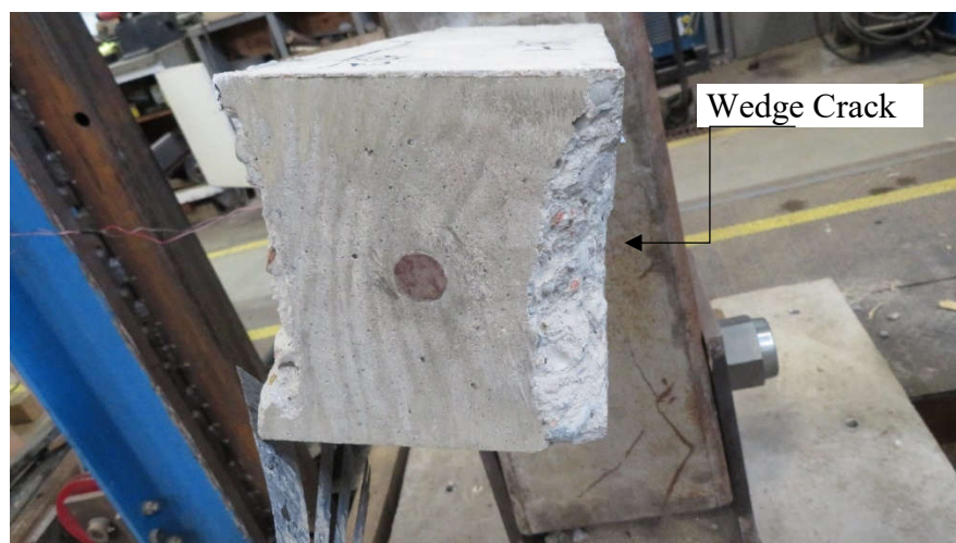
a) Wedge cracks formed after dynamic testing.
