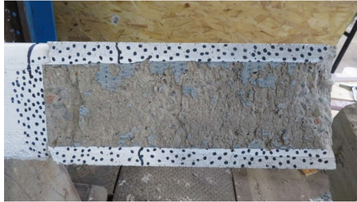
a) Dynamic test with mainly concrete failing.
