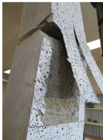
c) Typical static test with concrete failing.
