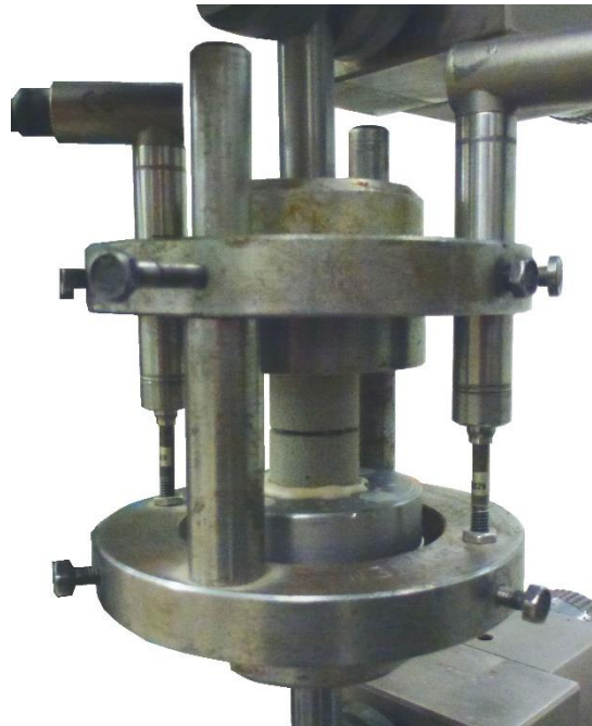
Fig. 1 — Quasi-static testing setup with a notched SHCC specimen
