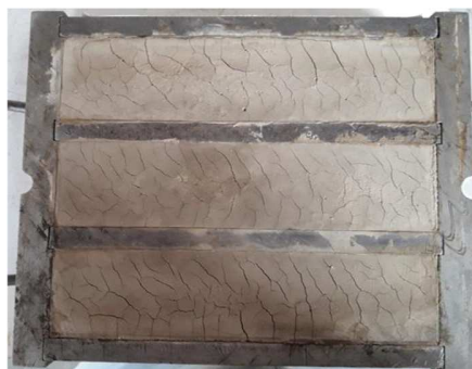
Fig. 1—Appearance of cracks just after setting for a cement paste with 2 wt% of humic substances and w/b=0.42 .
