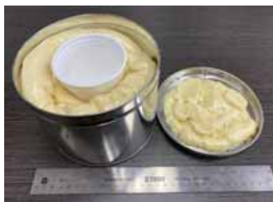
Fig. 7—Paint cans used for low-tech calorimetry experiments. Paint cans are filled with expandable foam to insulate it from exterior temperature. Mixed paste samples are placed in removable Styrofoam cups to facilitate easy sample preparation and cleanup following the experiment.
